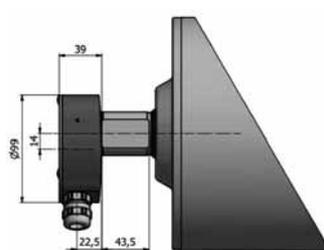
Terminal box in stainless steel  $\leq 4,0$  kW
