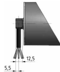
Cable slot 90° with threaded shaft
