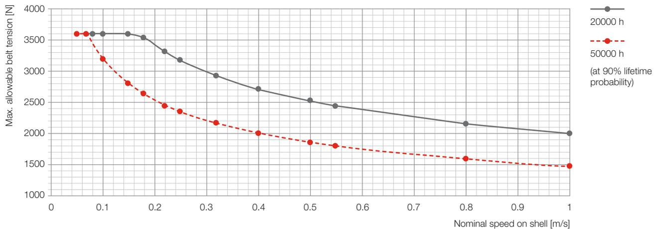
For the right allowable belt tension value please check the accordant nominal speed on the drum motor shell.
