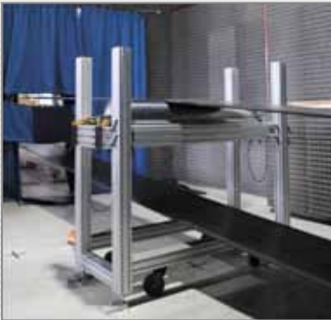
Rulmecca own measurement chamber, equipped with sound-absorbing materials
