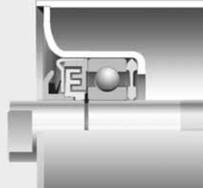
Section through sealing
