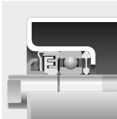
Section through sealing
