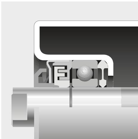
Section through sealing
