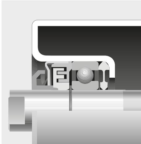
Section through sealing
