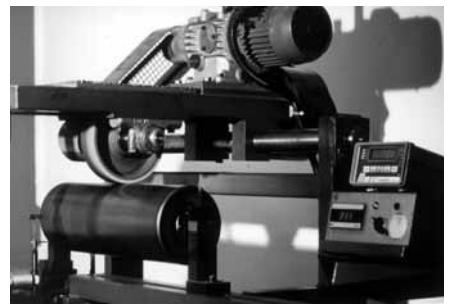
Machine for the dynamic hermetic test against water or dust ingress.
