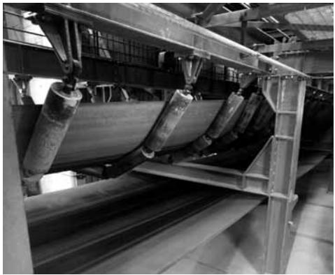
The diameters and types of rollers in the table are those advised for suspended sets with five rollers, for different widths of belt. The diameter of the roller is chosen from those possible for the type of roller considered (see chapter 2 rollers) and must be suitable for the speed and load capacity of the belt (see chapter 2 para. 2.3 selection method).
