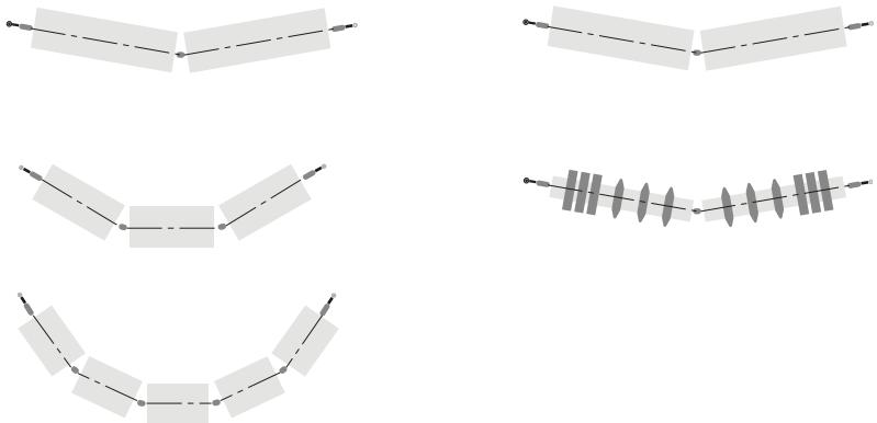
Fig. 8 - Suspended set for impact troughing set with three or five plain rollers or with shock absorbing rings
