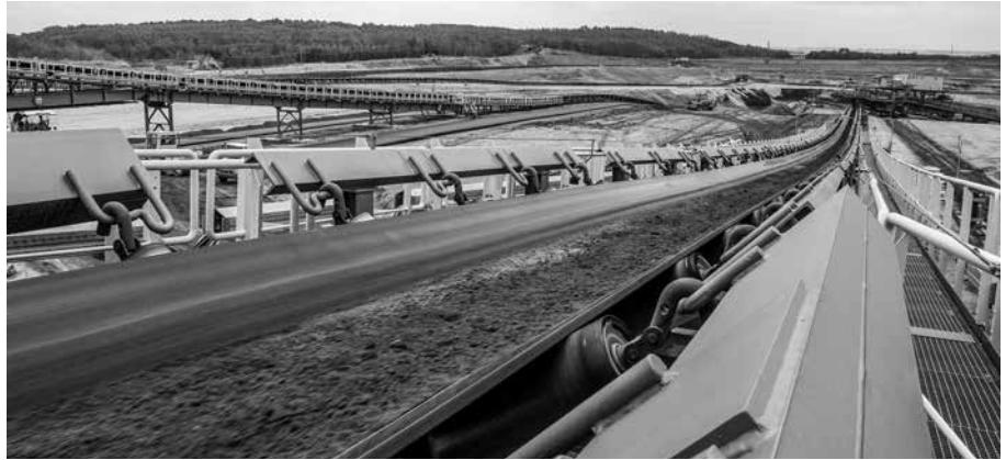
The residual material remains attached to the return section of the belt and may deposit onto the rollers in a non uniform way that promotes belt drifting and premature wear.
