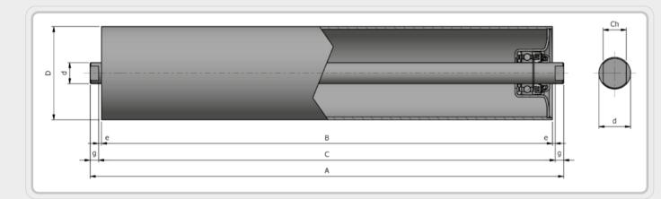
Idle rollers for heavy pallet conveyors in internal, external, normal, dusty and humid environments.
